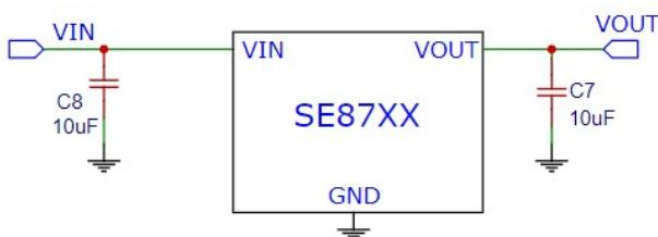
In plugging in application,  $C_{IN}$  is recommended to use  $10\mu F$  electrolytic capacitor or  $10\mu F$  MLCC with 2 ohm serial resistors to prevent large input voltage spike when plugging in. See APPLICATION INFORMATION for more information.
